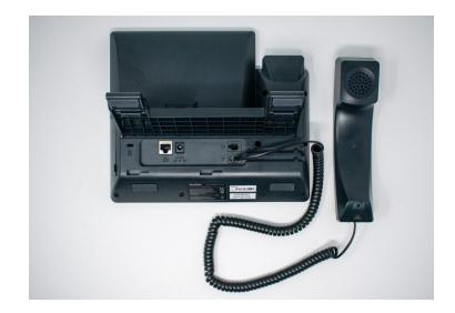
4. Plug in power cord to the port labeled DC12V.
